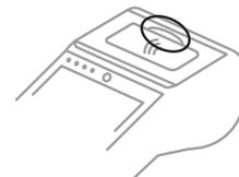
1. As shown below, pull up on the tab of the printing paper box cover to open it.
