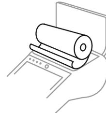
2. Load the printing paper roll into the printing paper box in the right direction as shown.
