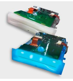
The AGE 300 reads magnetic, contact chip, and contactless ID cards. The AGE 300 can extract all data necessary to assess a user's birthdate and other relevant information. By inserting a card it is possible to read up to 3 magnetic tracks, asynchronous contact chip, and multiple protocol contactless chip. The AGE 300 supports USB, Serial and ccTalk protocols.
