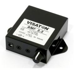
Stereo amplifier with level controls, e.g. for multimedia applications. Suitable for use with small loudspeakers with impedances of 4 to 8 ohms. Robust metal housing with two fixing lugs. Can be connected directly to the line out or headphones socket of a PC audio card, while the input sensitivity is regulated via the level control. Power supply (12 V) is via a mains adapter (not supplied) or the computer's on-board power supply. S h o r t - c i r c u i t p r o o f.
