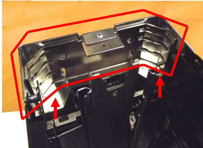
Additionally, inspect the housing cashbox cam located in the lock mechanism below the cashbox in the chassis for damage. If the cam is found to be bent or misaligned, a new housing cashbox cam must be ordered.
