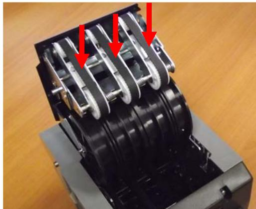
The same should be done to the three belts running inside the dispenser. They run through a set of three pulleys, one pulley per belt, and are located towards the back of the dispenser.
