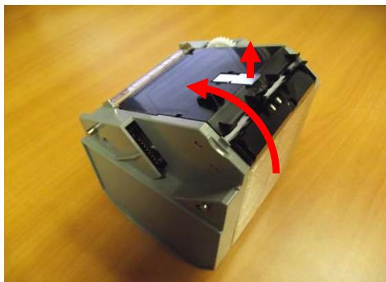
This reveals two sets of sensors, one at the edge of the cover, and the other at the edge of the recycling cassette. The two sets of sensors have to be cleaned using a cotton swab and then sprayed with compressed air to remove leftover loose dirt.
