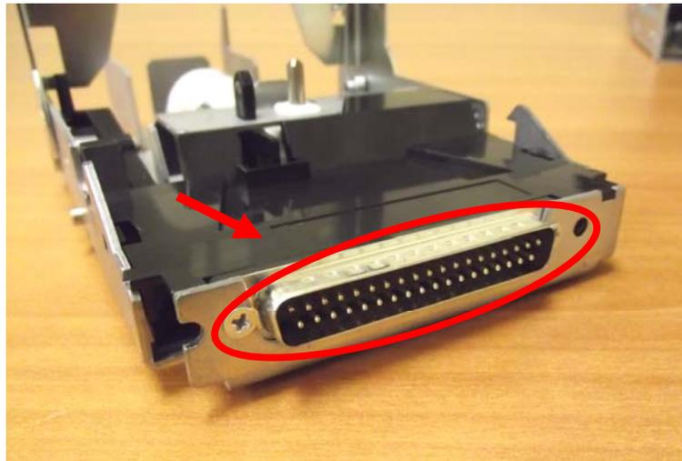
After the inspection has been performed, using a can of compressed air, spray the motor area, the connector and the rest of the surfaces to remove any excess dust. Then replace the power interface module back into the housing, completing Level 2 maintenance.
