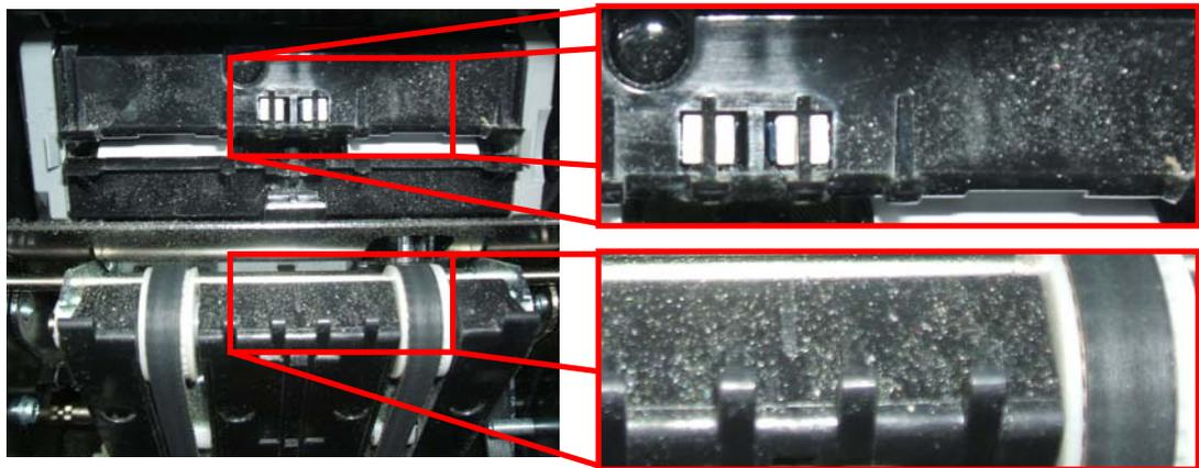
**Moderate** – The moderate level includes dust and debris that has been mixed with oily residue and requires additional effort in order to remove it from the surface (this can be seen mainly on rollers which place the dirt under pressure causing it to compact on its surface)
