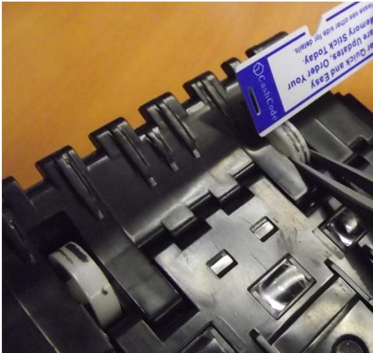
The o-rings are then cleaned using the alcohol-free LCD cleaner. Spray the antistatic microfiber cloth sparingly and wipe the o-rings. For best result, move the cloth in a direction perpendicular to that of the direction of rotation, turn the wheel and repeat.
