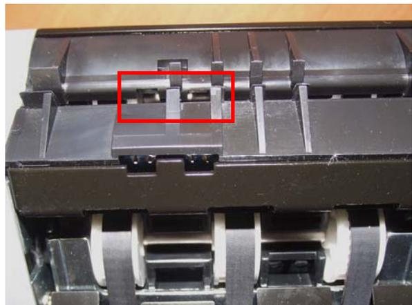
After the three sensors were cleaned, use a can of compressed air to spray around the sensors and spray any loose debris out of the dispenser. Ensure the dispenser cover is opened to allow excess debris be evacuated.
