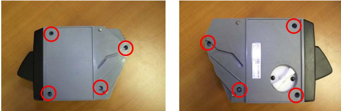
Remove the cover slowly to ensure no internal components are moved and connectors unplugged inside the dispenser.
