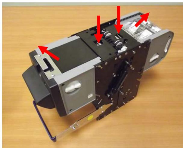
Open the chassis to reveal the bill path by pressing down the two latch buttons at the top face
