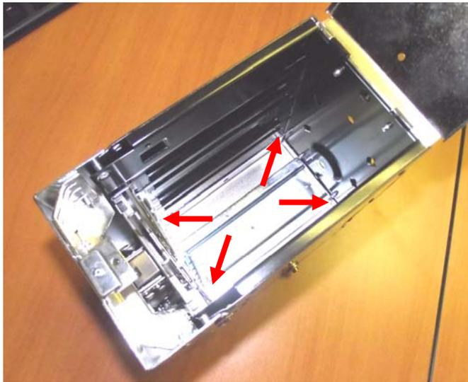
Next, use a lint-free microfiber cloth to wipe all surfaces and to ensure all oily residue and tough debris has been removed.
