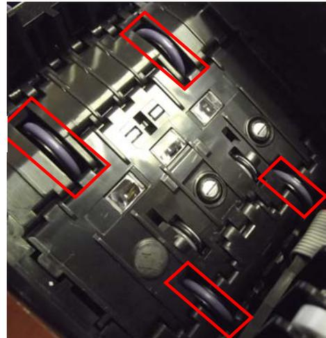
As the o-rings are being replaced, ensure the aligning mechanism worm gears are not damaged and clean them using a can of compressed air.
