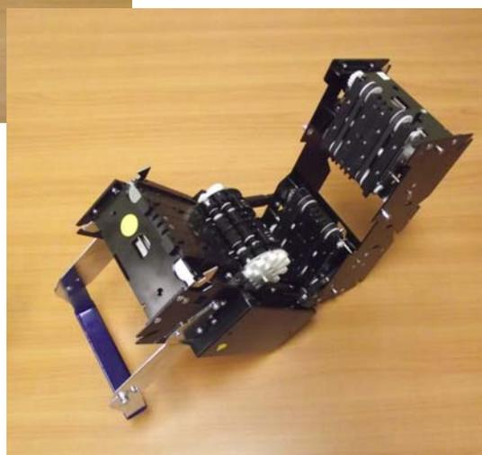
Each half of the chassis consists of 6 sets of bill position sensors distributed along the bill path. The sensors on one half can be distinguished by their clear rectangular appearance, and the sensors on the other half are clear circular lenses embedded in the body. These 12 sets of sensors have to be cleaned using a new cotton swab.
