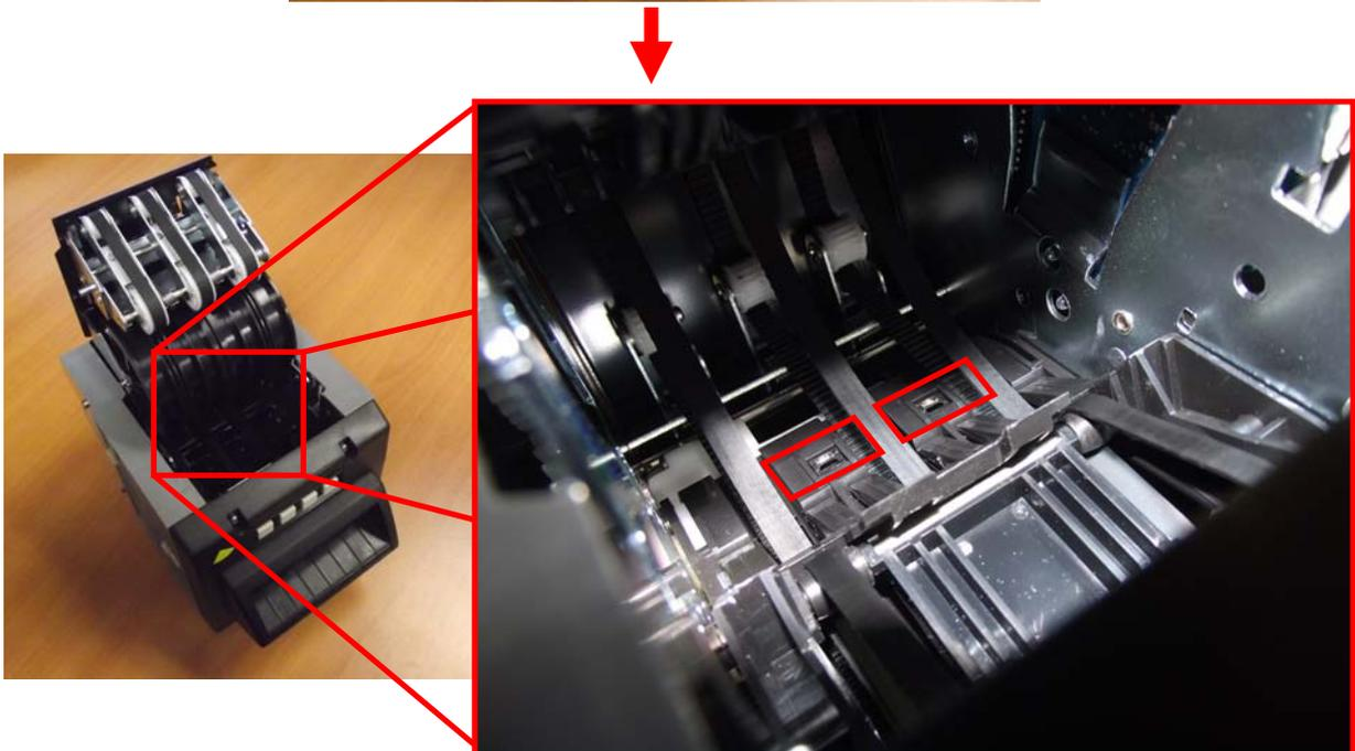
The third sensor is located at the bill entrance (entrance of the bill from the path switch). It should be cleaned using a new cotton swab
