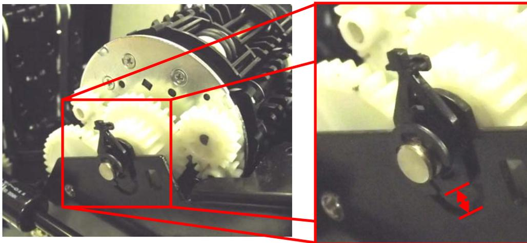
Ensure the switch itself is inserted into the chassis by the bearings to allow the free rotation of the switch. This will allow the switch to self-adjust in order to mesh with the gears properly and ensure no gap remains between the bearing and the groove in the chassis.
