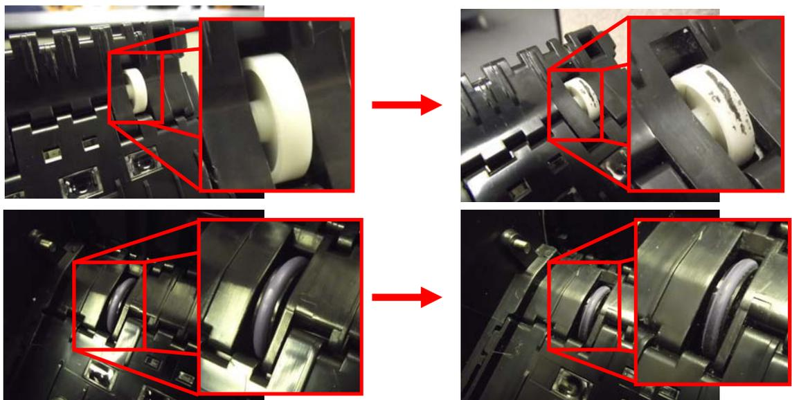
**Extreme** – Extreme dirt and debris cannot be removed without damaging the part. It has fused with the part or is located in an area that cannot be reached and therefore the part must be replaced in order for the Bill-to-Bill™ unit to function properly.
