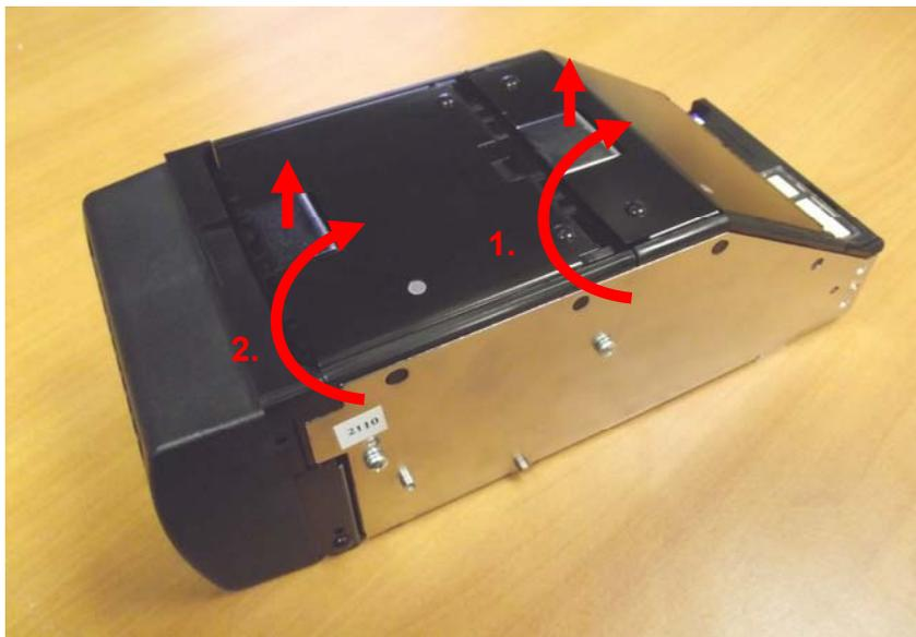
When trying to open the upper compartment, the motion is being restricted by a latch on the right side of the validator head (in a position where the front is facing the operator). The latch should be pressed inwards to allow the upper compartment to open up fully for easy access to the sensors.
