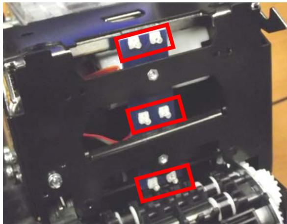
Some models may have plastic push rivets holding the guide assembly instead of screws as mentioned above. In order to remove the push rivets, several additional steps must be taken as follows:
