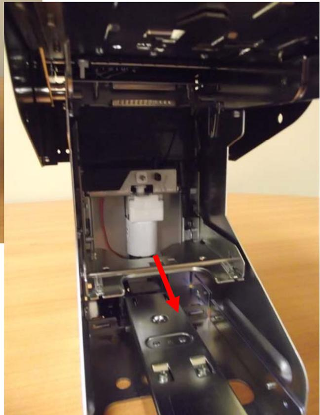
After the interface has been removed, check to ensure the two touch sensors are working properly by pressing them and ensuring they go back to their original position after they have been released.
