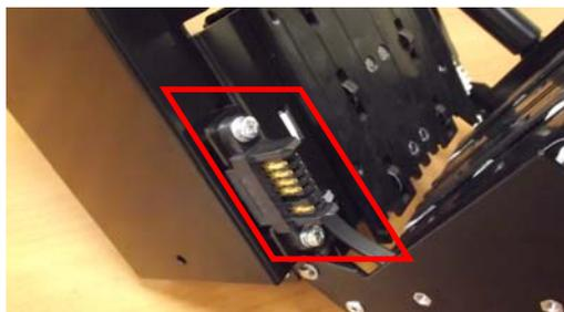
Once the maintenance has been completed for the Bill-to-Bill™ 300 chassis, re-insert the recycling cassettes and dispenser, and slide it back into the housing and ensure the locks holding the chassis inside are locked properly. If the lock does not fully engage, contact a certified technician for further analysis
