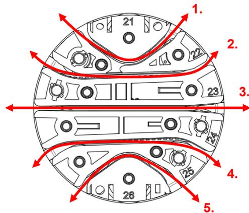
Once the card is inside, fix the switch so it will not move and using one hand on each side of the card, slide it sideways back and forth to properly clean the belts. Repeat the above steps for all 5 slits.
