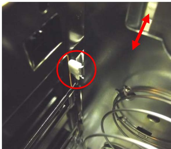
Using a can of compressed air, clear out any dust that might have accumulated at the back of the cashbox along the tracks of the bill stacking mechanism to ensure the cashbox reaches its maximum bill capacity.
