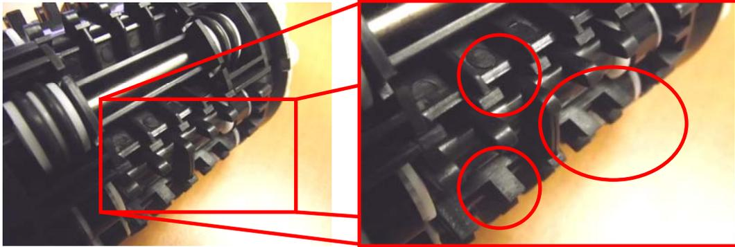
Also ensure that the switch lock works properly by first depressing it and then releasing it. The lock should snap back into its original position..
