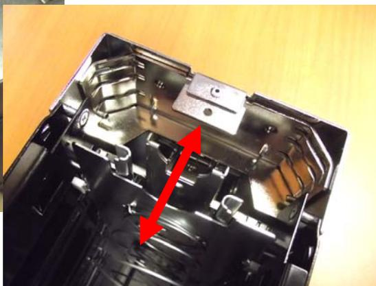
Visually inspect the cashbox cam used to lock the cashbox and ensure it is straight. Bend cams will compromise the security of the cashbox and must be checked often and replaced immediately if damage is detected (5106025).
