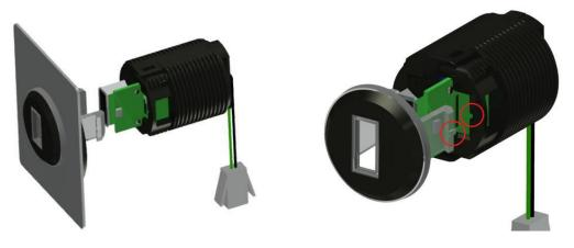
3. Move the housing with the PCB in a straight line towards the snappers of the cover. Align the housing side with the groove to the snapper with the lip.
