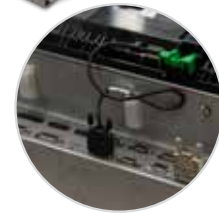
Dongle contains the software and configuration for the CAM is included
