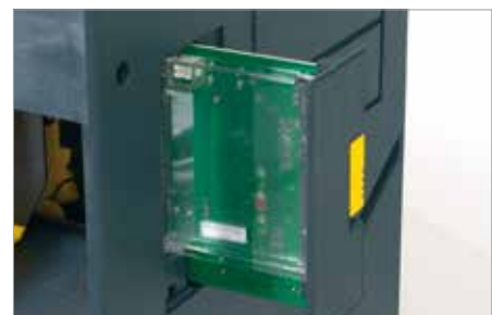
Board easily extractible from the outside
