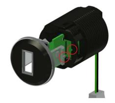
3. Move the housing with the PCB in a straight line towards the snappers of the cover. Align the housing side with the groove to the snapper with the lip.
