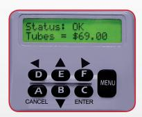
Keypad and LCD display for quick and simple navigation
