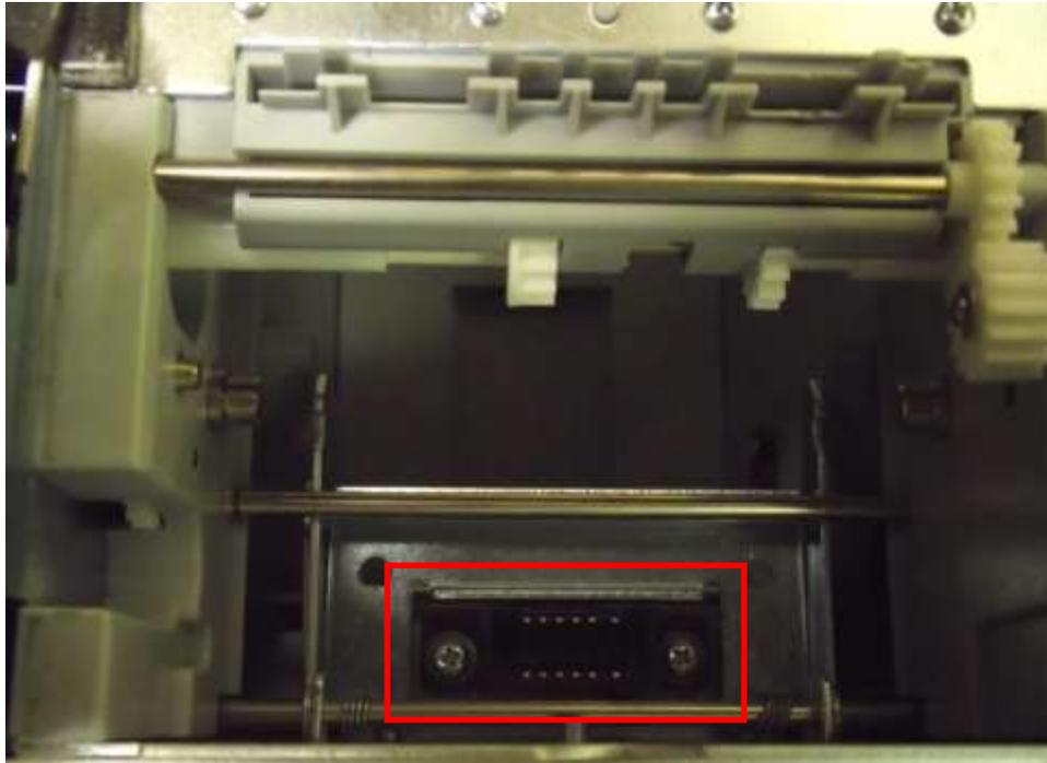
After the inspection has been performed, using a can of compressed air, spray the motor area, the connector and the rest of the surfaces to remove any excess dust. Then replace the power interface module back into the housing, completing Level 2 maintenance.
