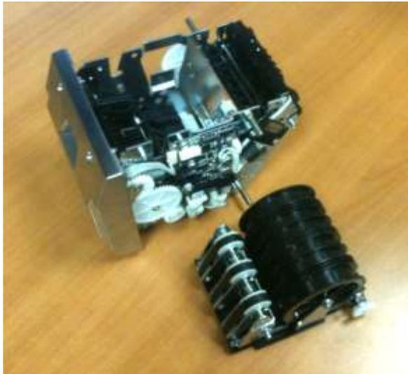
More importantly, the belts are cleaned using the LCD cleaner and an anti-static microfiber cloth. The belts can be manually rotated and cleaned all round.
