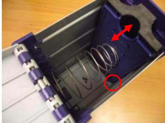
Using a can of compressed air, clear out any dust that might have accumulated at the back of the cashbox along the tracks of the bill stacking mechanism to ensure the cashbox reaches its maximum bill capacity.
