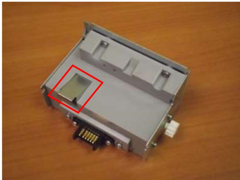
Also, ensure that the connector inside the box control unit compartment on the chassis is not damaged and that all the pins are straight to ensure proper communication between the housing and the cashbox.
