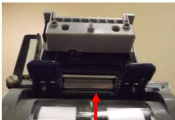
After the bill validator has been removed, open the lower and upper compartments.
