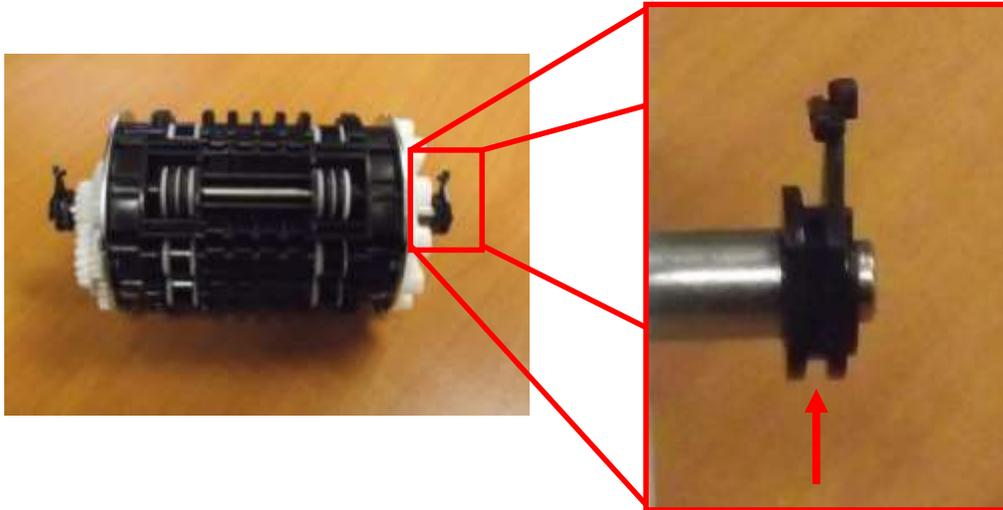
The groove on the bearings should be placed onto the body of the chassis.
