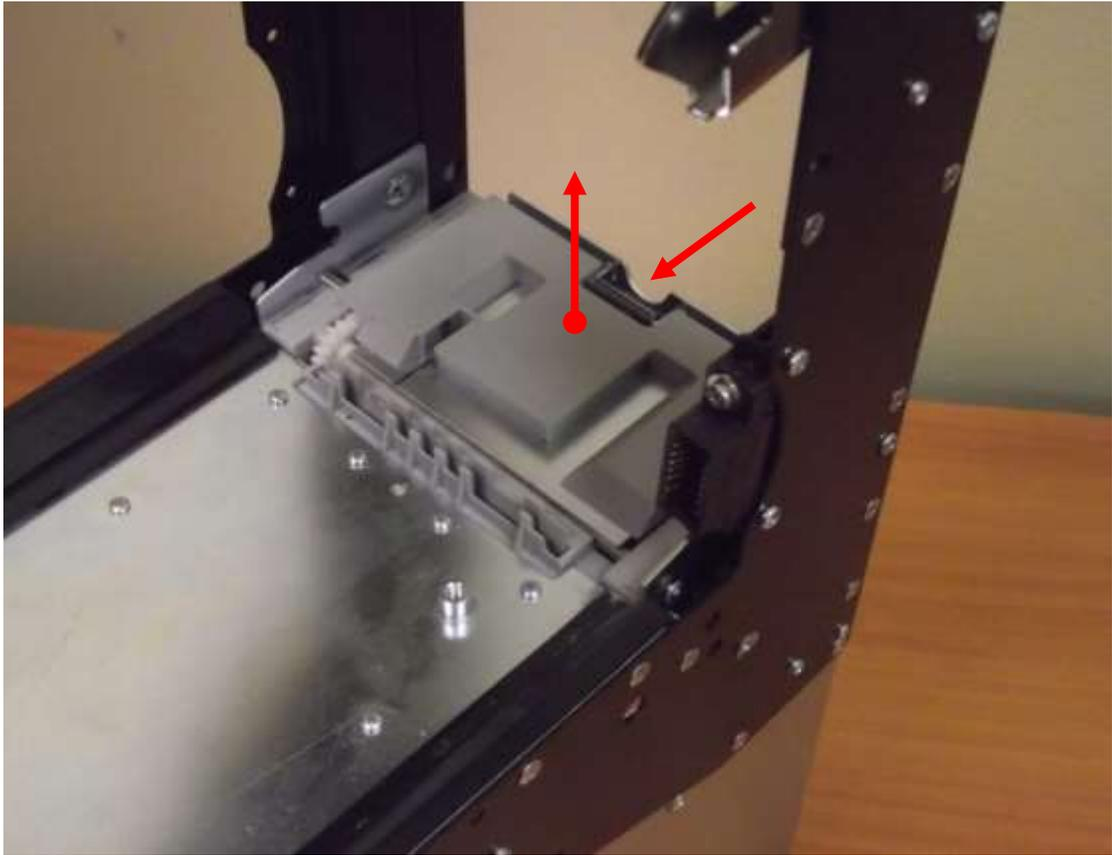
After the interface has been removed, check to ensure that the main connector does not have too much play about it and none of the teeth on the motor gear are chipped or broken.
