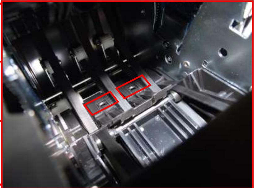
The third sensor is located at the bill entrance (entrance of the bill from the path switch). It should be cleaned using a new cotton swab
