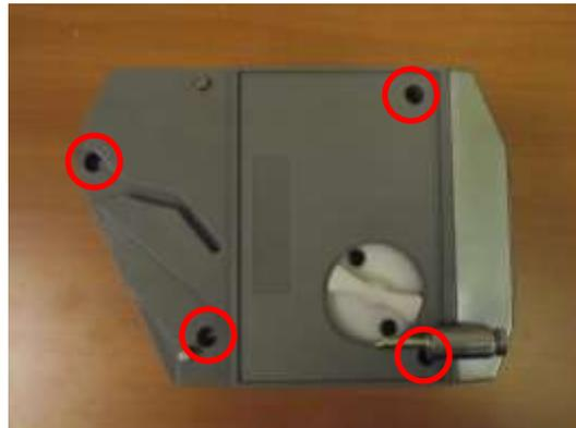
Remove the cover slowly to ensure no internal components are moved and connectors unplugged inside the dispenser.
