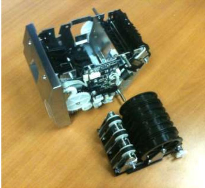
Optional: Turning the dispenser over would reveal the shutter and drive motors. It is recommended to replace these motors during Level 3 maintenance at **540,000** cycles (0300052-02).
