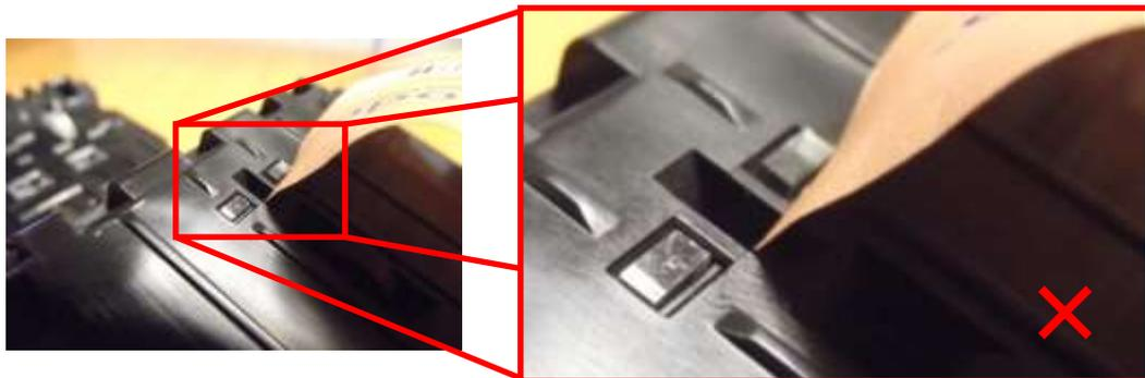
The rollers however should be cleaned more thoroughly in order to remove the oily residue and debris that is stuck to its surface. Each roller, at its turn, should be held in place by a pair of tweezers and using the Suzo-Happ Group dummy card, all the black and/or green dirt should be removed.
