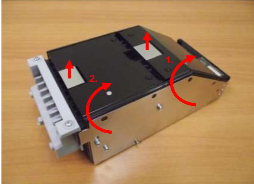
When trying to open the upper compartment, the motion is being restricted by a latch on the right side of the validator head (in a position where the front is facing the operator). The latch should be pressed inwards to allow the upper compartment to open up fully for easy access to the sensors.
