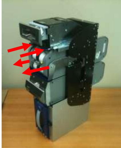
Next, remove the recycling cassettes and dispenser by pressing the release button of each module and pull it away from the chassis. Set the module aside.
