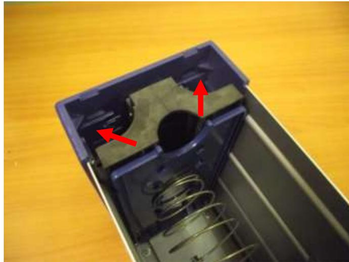
Additionally, inspect the housing of the cashbox. Visually verify that the cable harness does not have damaged wires, the red security switch springs back when it is pressed and none of the other metal parts are bent.
