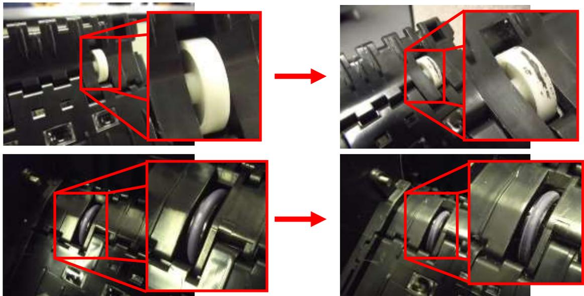
**Extreme** – Extreme dirt and debris cannot be removed without damaging the part. It has fused with the part or is located in an area that cannot be reached and therefore the part must be replaced in order for the Bill-to-Bill™ 300XE unit to function well.
