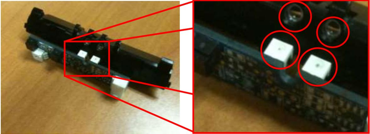
Turning around the PCB board would reveal two additional sensors which must be cleaned using a cotton swab. Use a can of compressed air to remove dust from the rest of the part.
