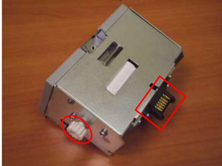
Turn the module around and verify the main latch is not bent and it springs back to its original position once it is pressed and released.
