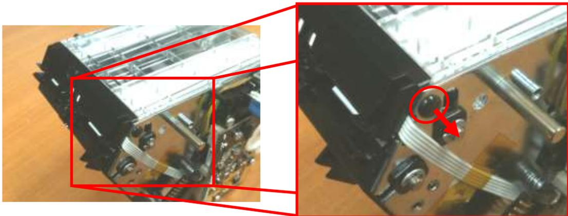
After removing the sensor array, remove the plastic push rivet securing the PCB and using a cotton swab, clean the two white light sensors and their respective lenses.
