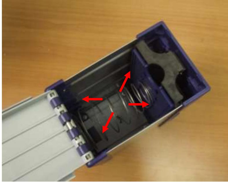
Next, use a lint-free microfiber cloth to wipe all surfaces and to ensure all oily residue and tough debris has been removed.
