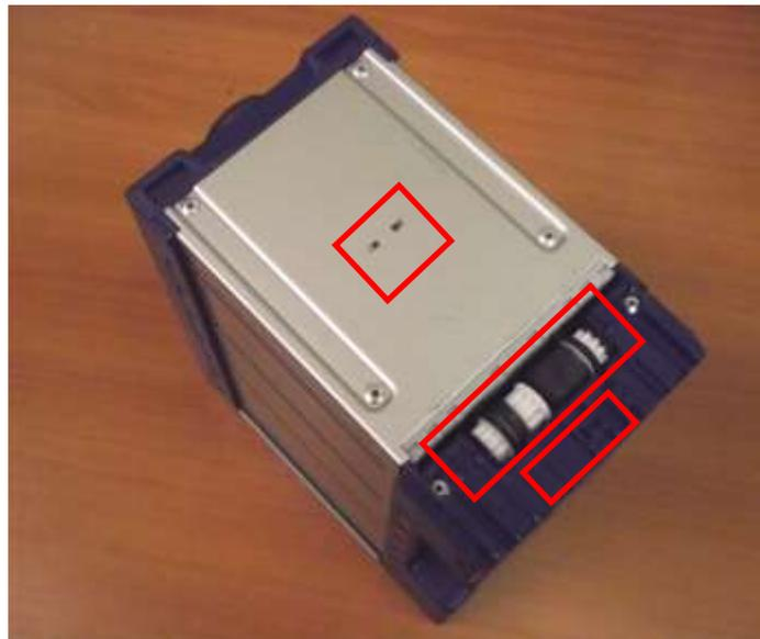
Visually inspect the cashbox cam used to lock the cashbox and ensure it is no broken and does not show any attempts of vandalism. Damaged cams will compromise the security of the cashbox and must be checked often. Replace cashbox immediately if damage is detected.
