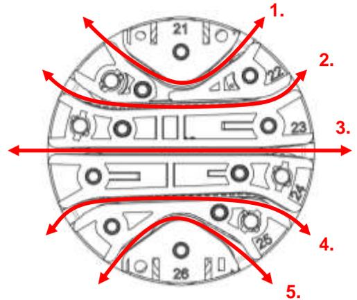
Once the card is inside, fix the switch so it will not move and using one hand on each side of the card, slide it sideways back and forth to properly clean the belts. Repeat the above steps for all 5 slits.
