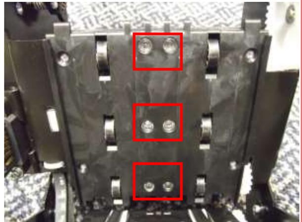
Then, using a can of compressed air, spray the bill path (sensors and rollers) on the two halves of the chassis.
