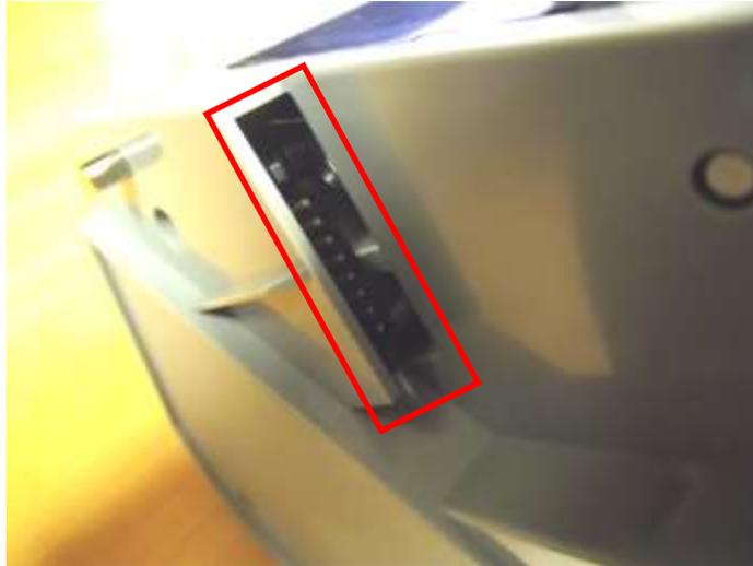
If any damage is detected, replace the connected along with the connector wire (0500109) by removing the two side covers of the cassette and unclipping the wire.
