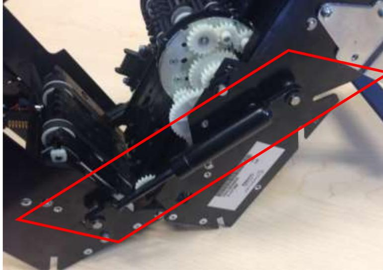
When reinstalling the gas piston, the orientation of the spring is essential and the rod side must be installed downwards away from the switch as seen in the image above.
