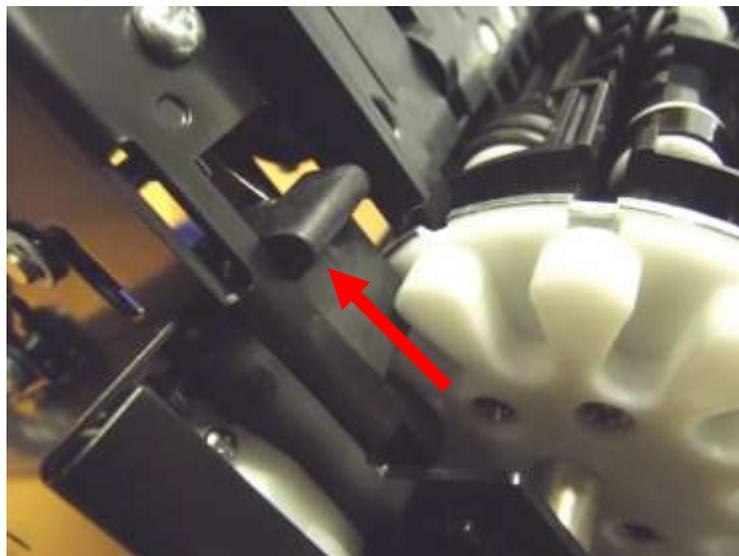
After the switch has been removed, using a can of compressed air, spray each slit thoroughly. Also spray all other surfaces including the gears end and the stepping end (index disk) of the switch. This will prevent the dust from wearing the surface of the teeth on the gears and that of the index disk.
