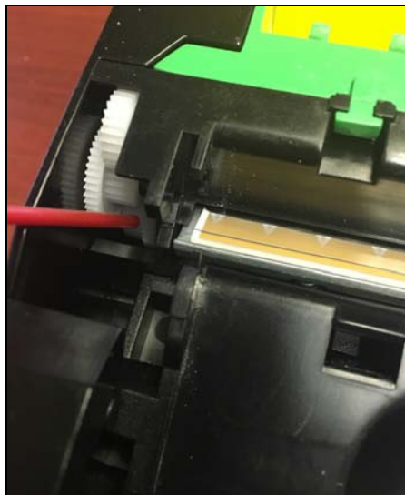
Figure 41: Clear dust off gears using compressed air
