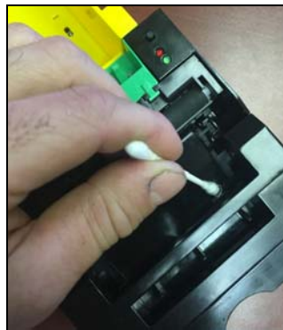
Figure 40: Clean paper guide sensor using cotton swab
