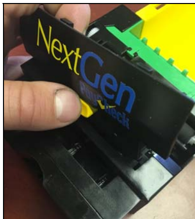
Figure 37: Remove top paper guide
