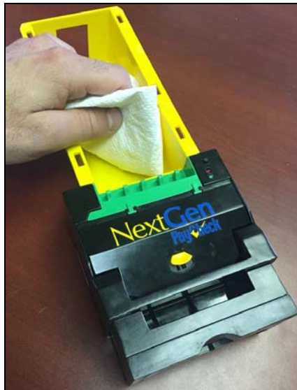
Figure 36: Remove excess dust
