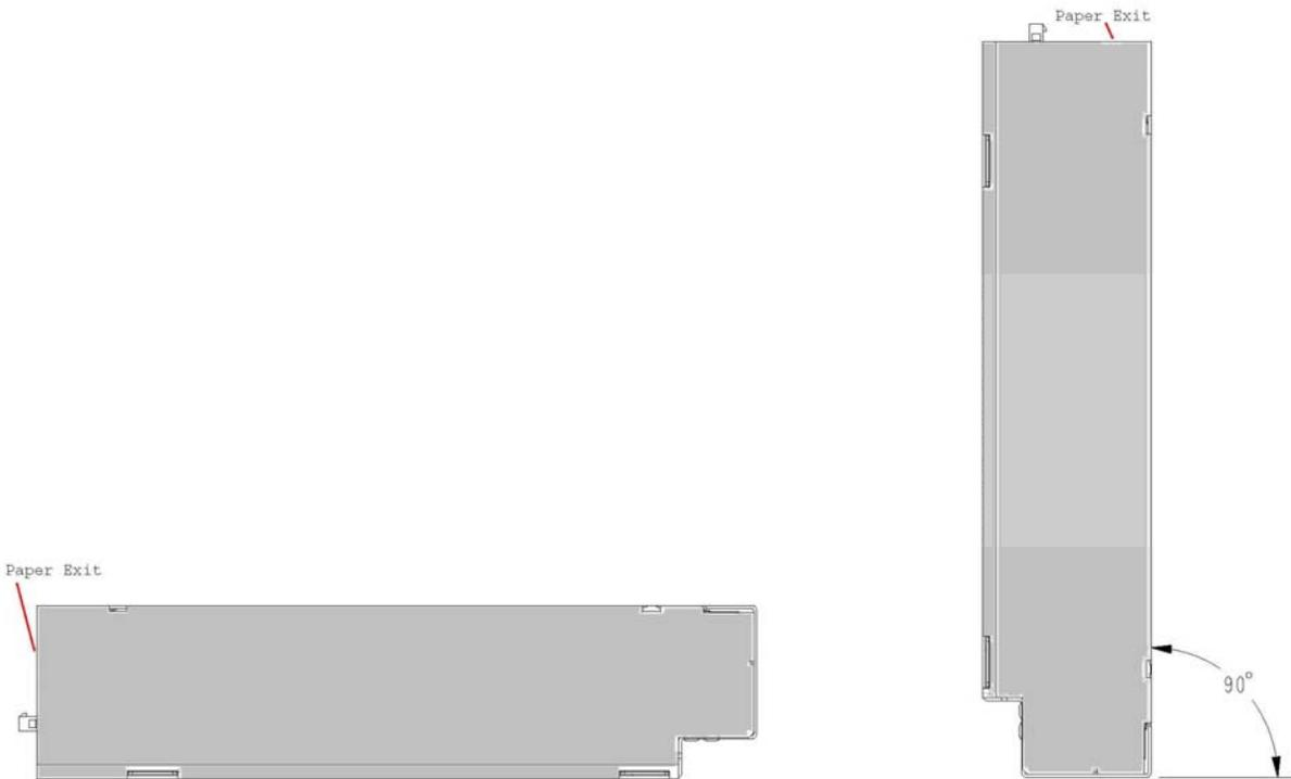
**Figure 6: Horizontal and Vertical Mounting positions**
