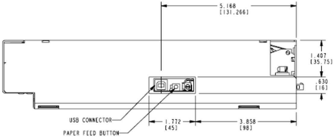
**Figure 15: Mechanical Dimensions – Paycheck 4™ Printer Left Side View**
