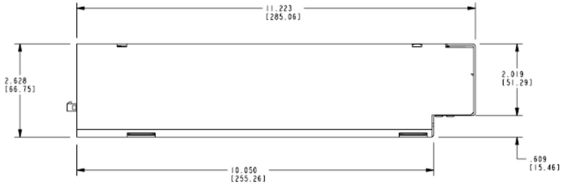
**Figure 11: Mechanical Dimensions – Paycheck 4™ Printer Right Side View**
