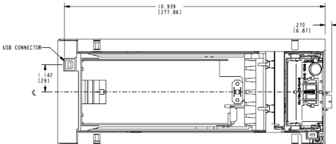
**Figure 14: Mechanical Dimensions – Paycheck 4™ Printer Top View**
