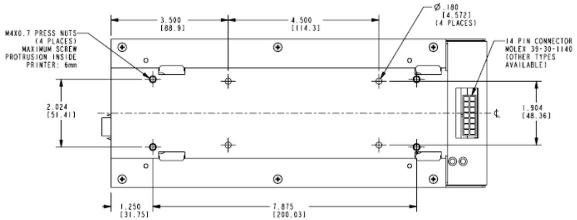
**Figure 12: Mechanical Dimensions – Paycheck 4™ Printer Bottom View**
