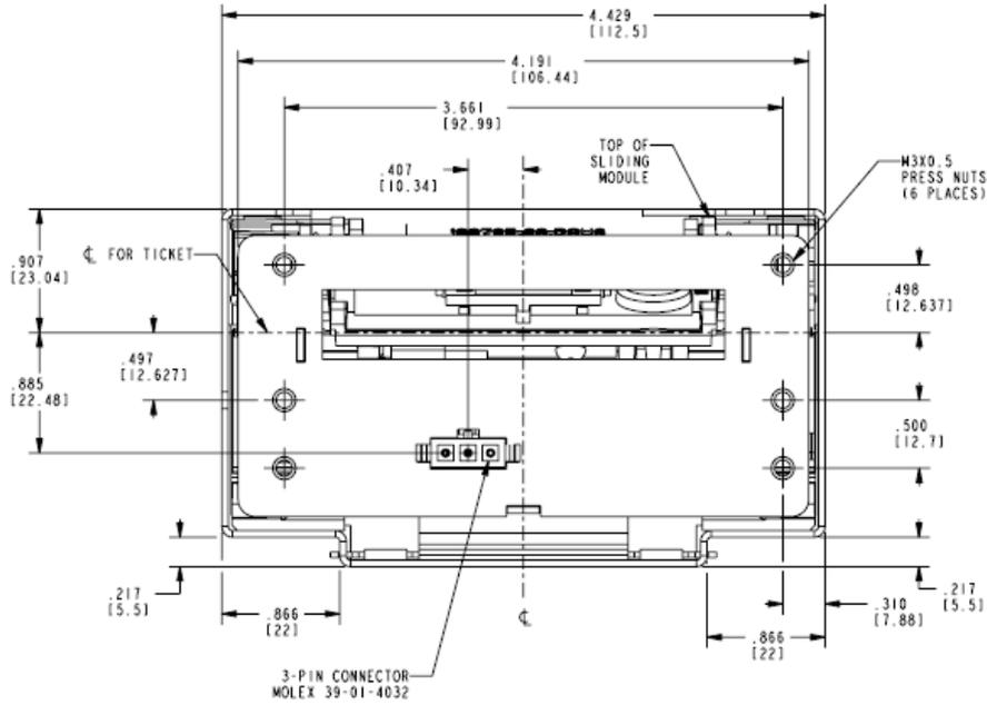
**Figure 13: Mechanical Dimensions – Paycheck 4™ Printer Front View**
