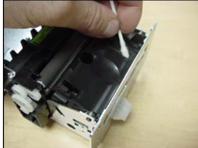
Figure 39: Clean paper guide sensor using cotton swab
