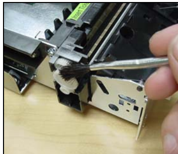
Figure 41: Clear dust off gears using light brush
