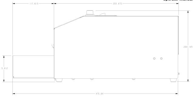
Figure 16: Side View with Cover Closed (in mm)
