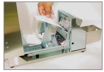
3. Lift the top ticket from the stack and align the left edge of the ticket to the left edge of the input paper guide.
