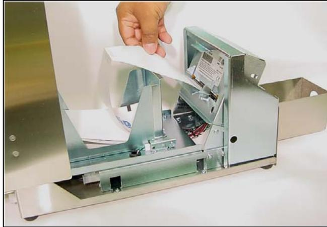
**Figure 3: Aligning Paper Edge**
