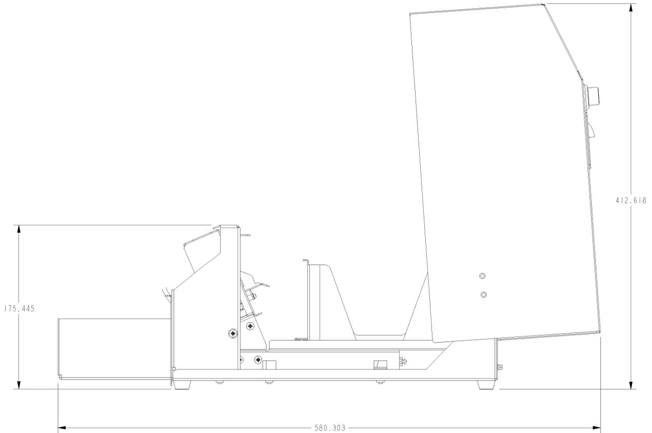
**Figure 15: Side View with Cover Open (in mm)**
