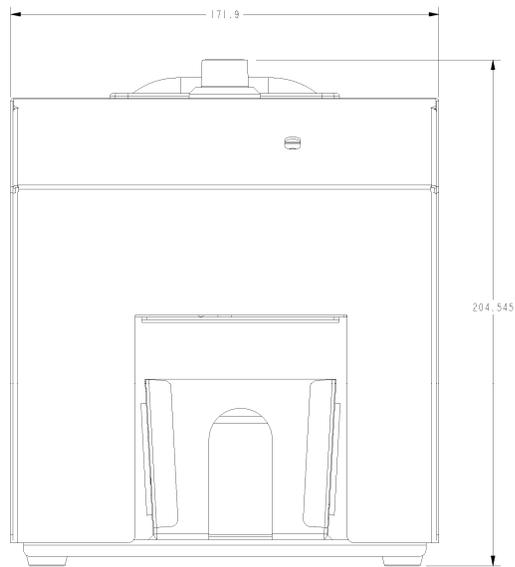
**Figure 17: Front View with Cover Closed (in mm)**
