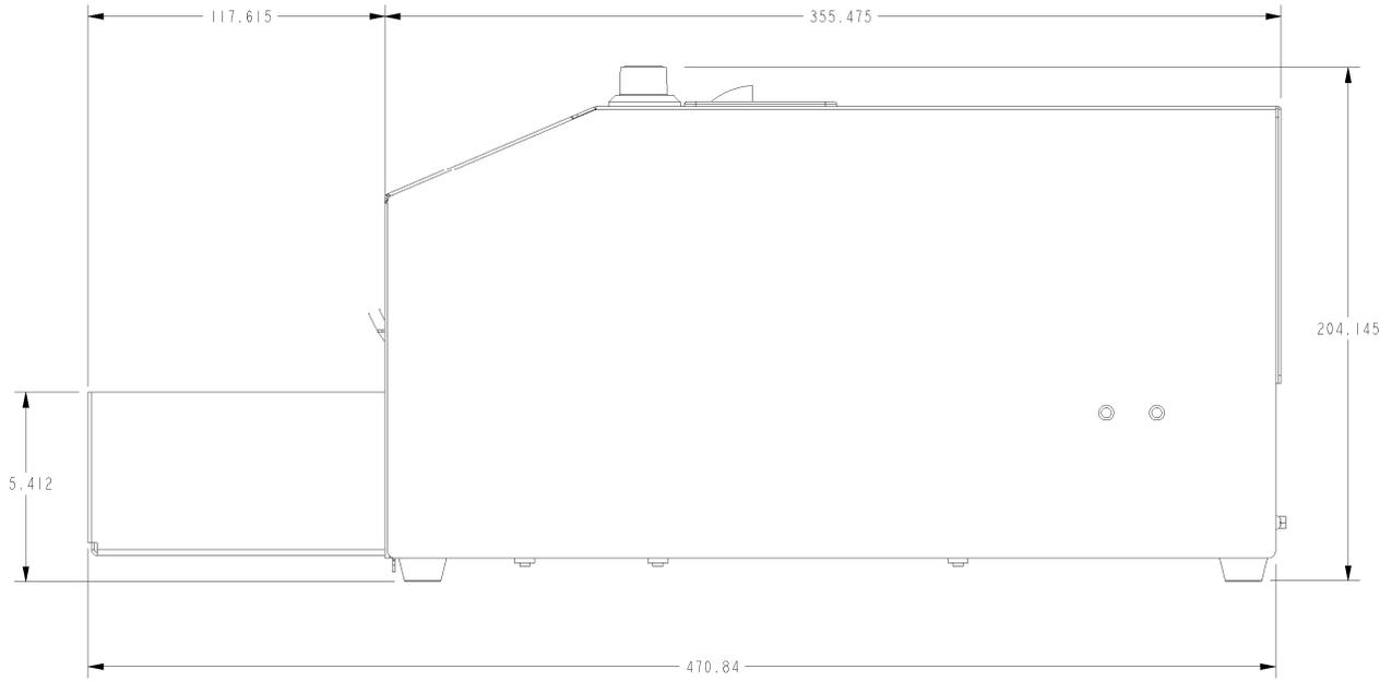
**Figure 16: Side View with Cover Closed (in mm)**
