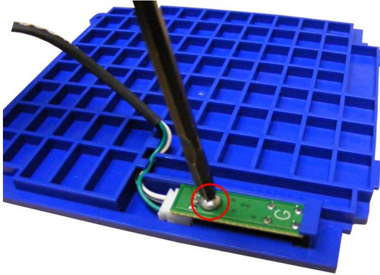
Figure 22: Main Board Screw Location
