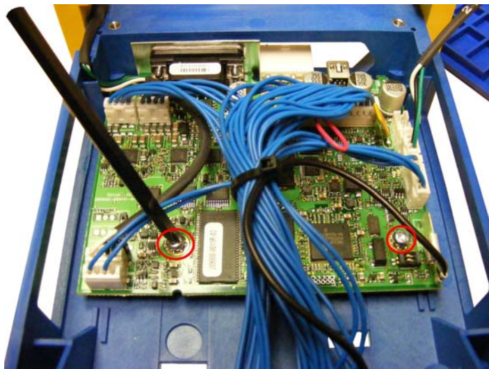
Figure 21: Main Board Screw Location
