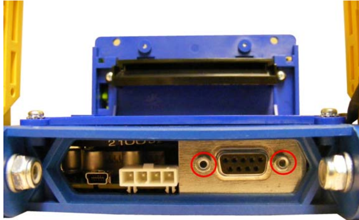
Figure 20: DB9 Screw Location
