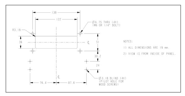
Install the **Optional Front Face Plate** for the wooden panel from outside the cabinet using four M6 (or 1/4 inch) carriage bolt.
