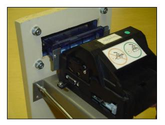
The **EZ-Tear Printer** can be adjusted to different panel thickness by sliding the four screws in the slotted base.
