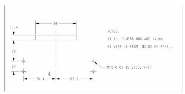
Secure the **EZ-Tear Assembly** through the four clinch studs on the metal panel using four M5 (or #8) lock nuts.
