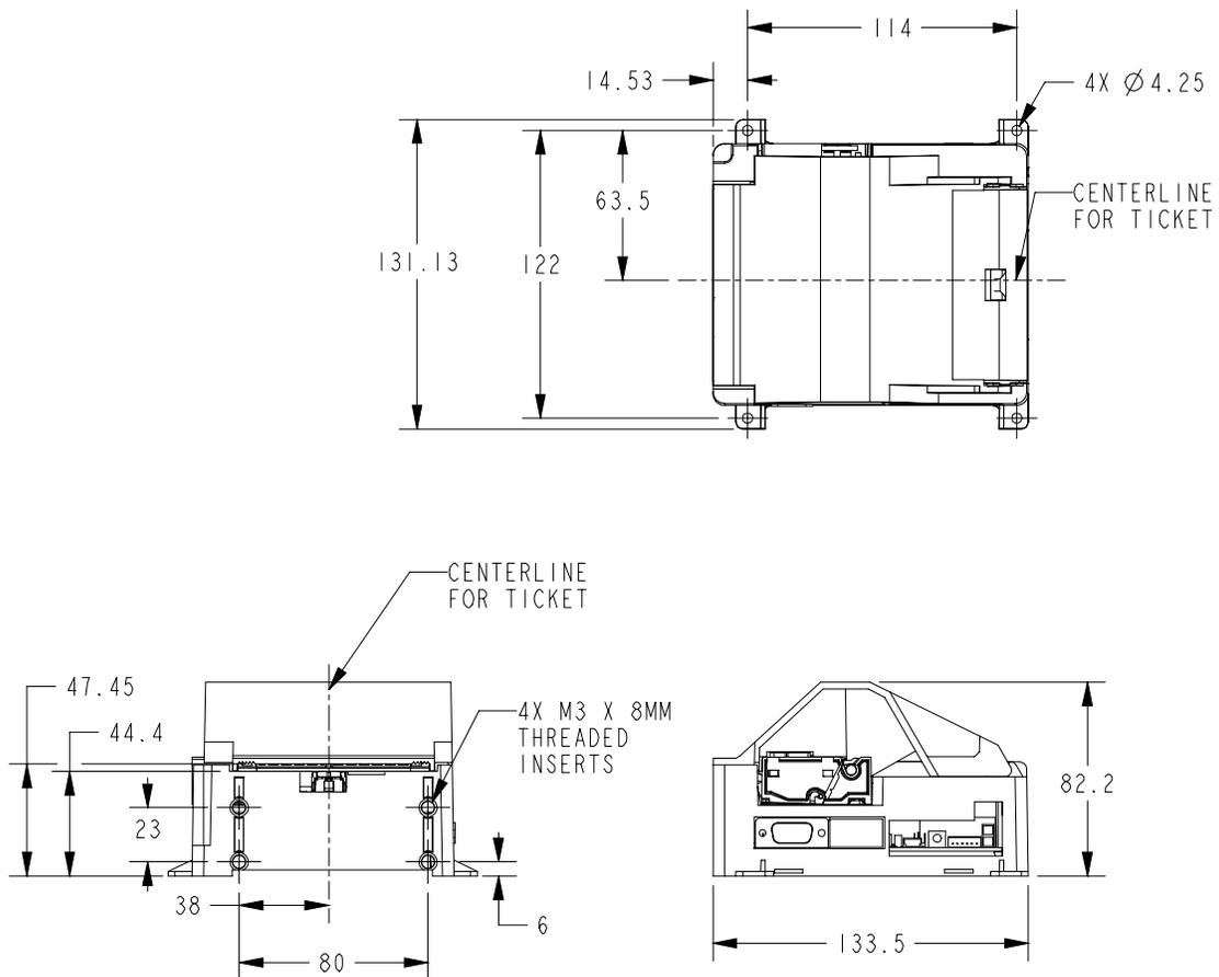
**Figure 8: Mechanical Dimensions**
