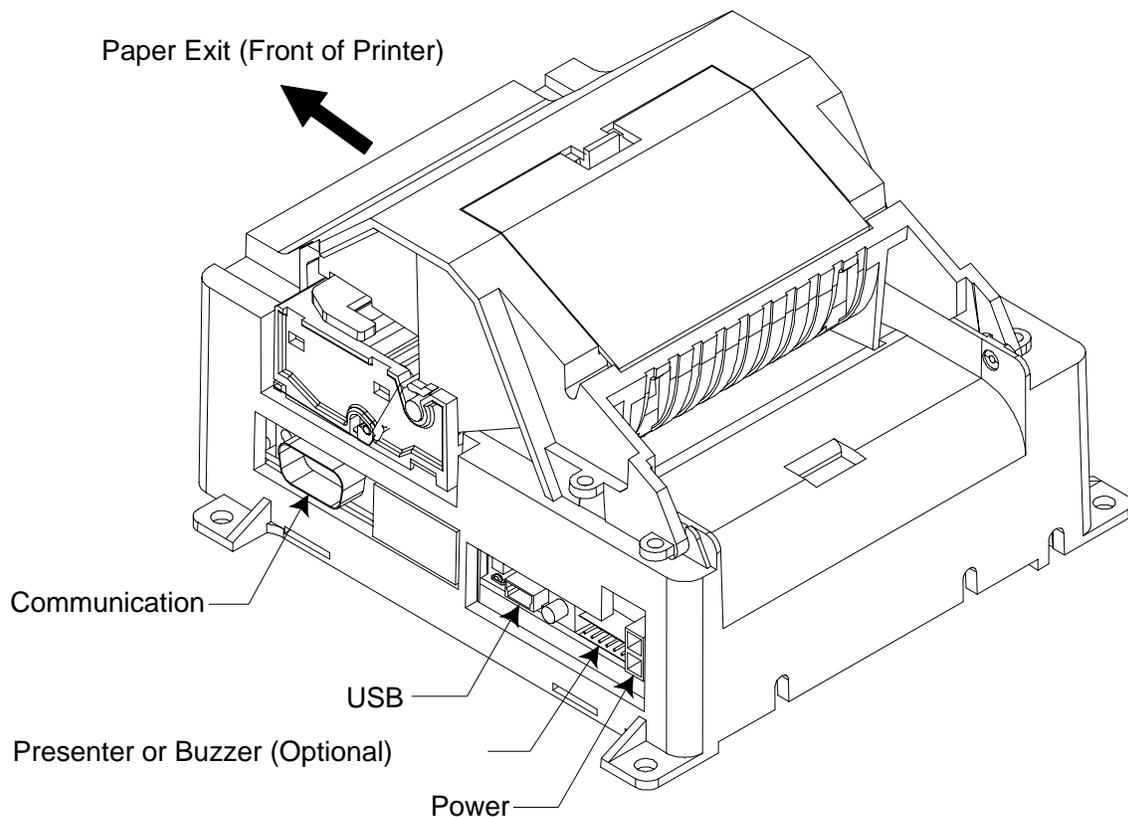
**Figure 2: Nanoptix EZ-Tear connection
