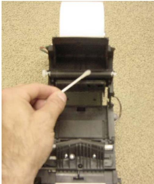
3. Clean the print line (black line on the print head) with a cotton swab and isopropyl alcohol.
