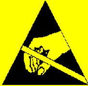
ESD protection (such as a wrist strap) must be used anytime a PCB is exposed
