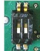
4. To avoid the HW watchdog from resetting the printer in the middle of flashing, temporarily remove the jumper SW101 (Note: This is optional because jumper not present on all board revisions)
