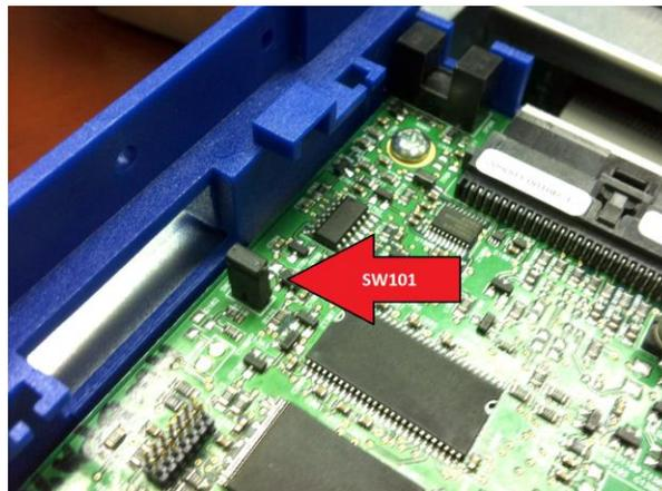
5. Then turn the printer’s power on. When the processor powers up and sees the two dip switches in the ON position it goes into an internal factory boot mode. After the printer is powered on, the dip switches need to be switched back to the OFF position.
